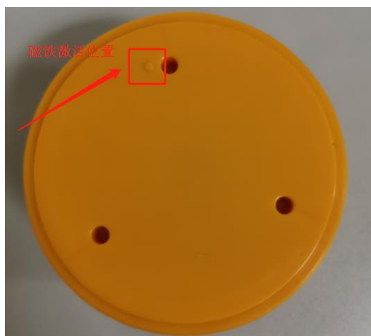
Figure 8. Marking at the magnet calibration position
