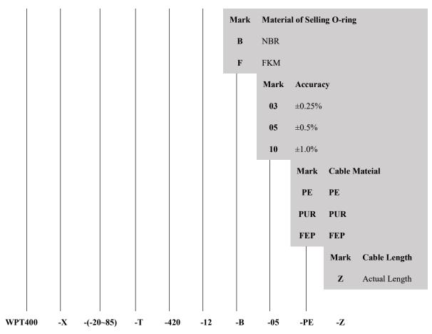
For example: CS-WPT400-5m-(-20~85)-T-420-12-B-05-PE-10m means:
