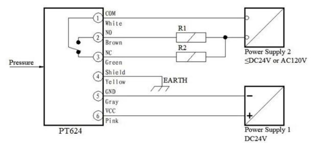
As shown above, the power supply 1 and 2 can be a same one, also can be unrelated. The power supply 1 is the power supply for this pressure switch. The power supply 2 is the power supply for the load, it should not exceed DC24V (or AC120V). The connection mode of the load is shown as R1 (or R2) in the figure. If the load requires the direction of the power supply (as current voltage), please follow the corresponding requirement.
