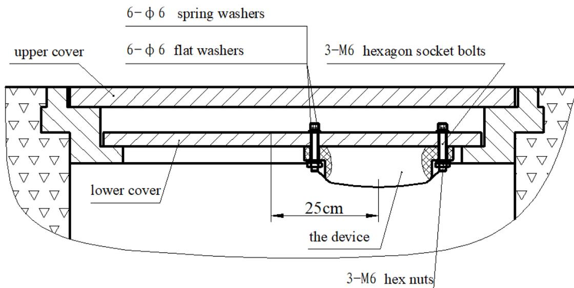
Figure 4 Installation instruction with CS-iTWM-A03
