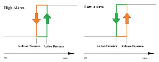
Return Stroke Error = | Action Pressure - Release Pressure |
