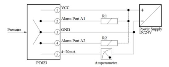
The load R1 (or R2) should be connected between the alarm port A1 (or A2) and VCC port. The action pressure of each alarm port can be set separately.
