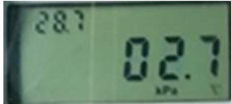
The temperature variable unit is Celsius ( $^{\circ}\text{C}$ ), and the data is displayed in the upper left corner of the liquid crystal. The pressure is in kilopascals (kPa) and the data is displayed in the middle of the panel.
