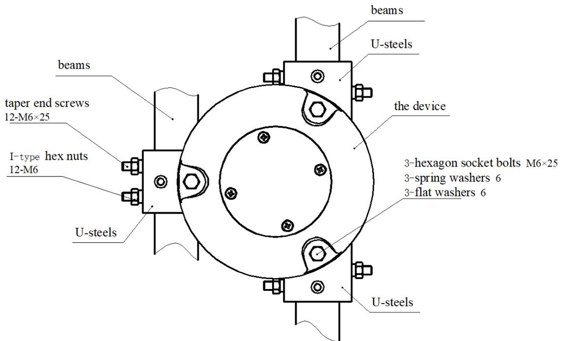
Figure 12 Installation Instruction with CS-iTWM-A02
