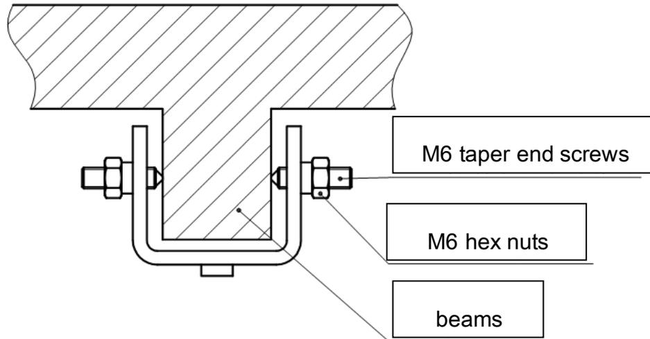
Figure 11 Installation instruction with U-steels
