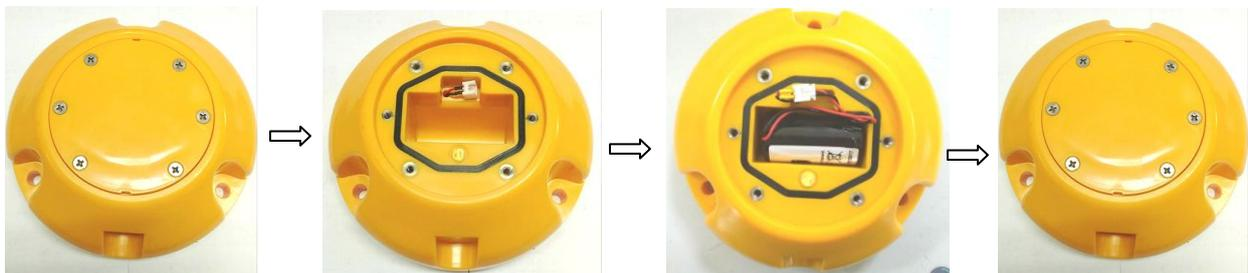
Figure 4 Battery installation or replacement
