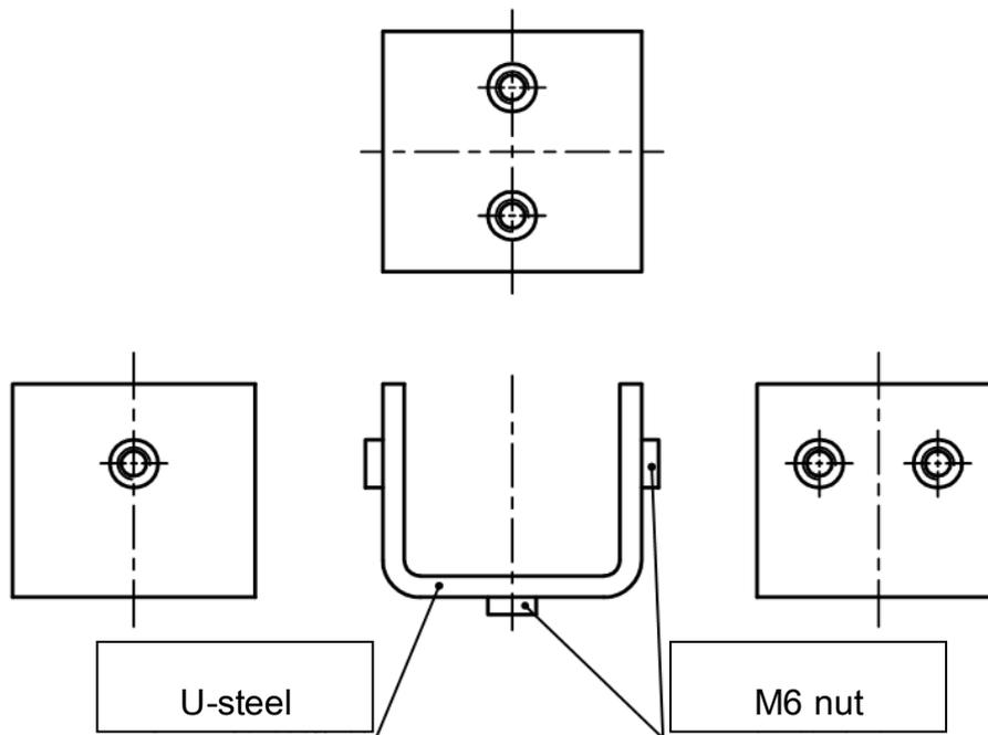
Figure 10 Installation instruction with rivet nut
