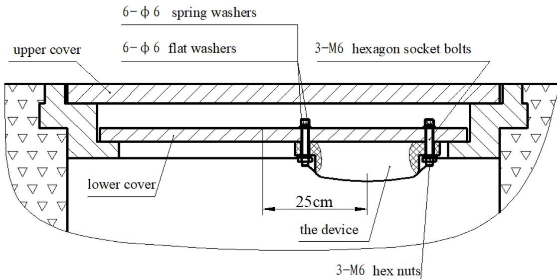
Figure 7 Installation instruction with CS-ITWM-A03
